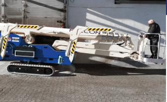
The Falcon Spider Atrium Lift is capable of passing through a door opening a mere 4'1" wide and 6 ft high.
