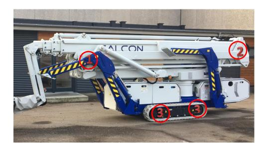
**Strap 1** - Strap the Falcon in the **rear end** by the fixing points and to a fixing point at the truck.
